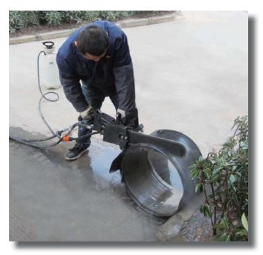
The APC42 Auto Pipe Cutter is designed specifically for cutting large pipe up to 1600 mm for municipal water repair. It is capable of cutting cast iron, ductile iron, and steel tube. The design allows for automatic cutting of the pipe with remote operation.
