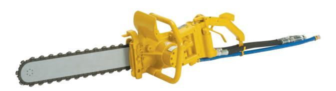
The **DS11** Diamond Chain Saw is specifically designed to cut solid concrete underwater. Cuts square corners without over-cut and can plunge cut sea walls up to 18" thick. Two available bar lengths (15" and 18") and two different chains depending on the amount of rebar and hardness of the concrete. A minimum of 20 PSI water pressure is required at the saw for cooling and lubrication of the bar and chain. Painted hi-visibility yellow.
