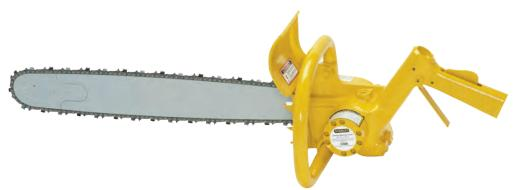
The **CS06** is a hydraulic powered chain saw for cutting all types of wood structures underwater - including bridge pilings, pier and dock timbers. It's compact design and high torque gear motor provides divers instant chain speed to cut through the toughest timbers with ease. The power to weight ratio is significantly higher than any other wood cutting chain saw and is available with bar lengths up to 20" (51 cm). Painted hi-visibility yellow.
