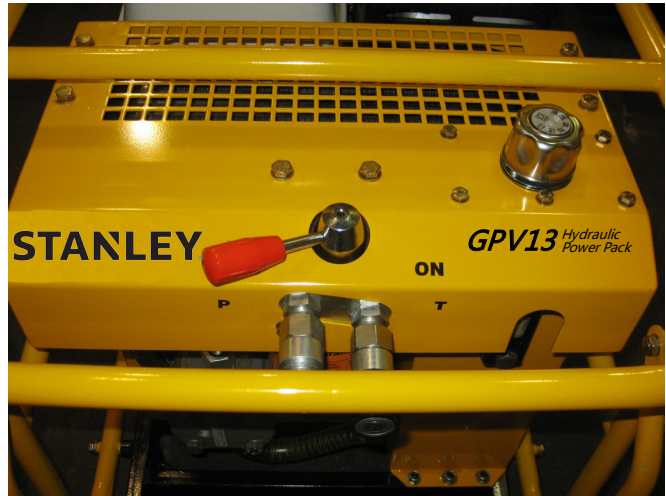
Figure 2. Panel Control Valve
