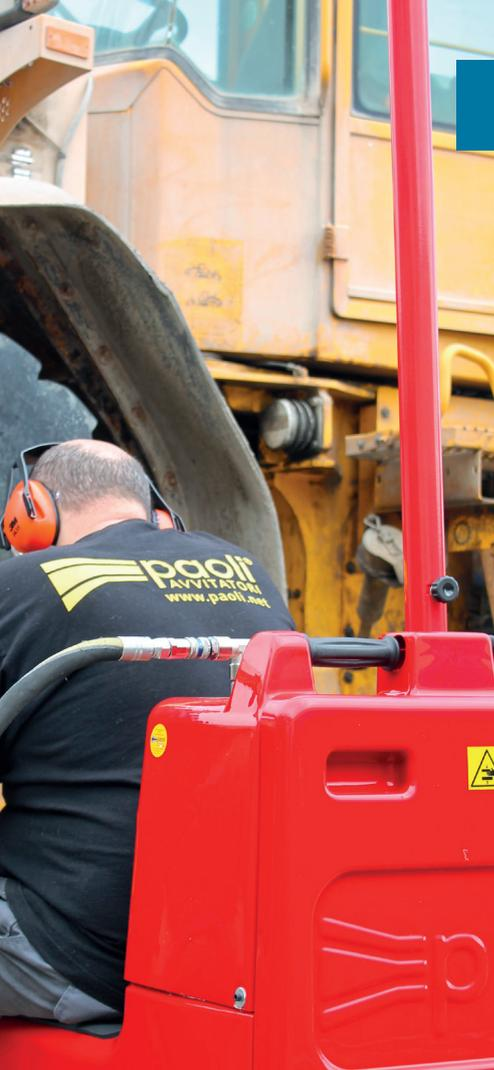
PAOLI has invented a mobile work unit in order to allow operators to work whilst comfortably and ergonomically seated and at the same time avoiding the necessity to hold the impact wrench constantly thanks to a built-in suspension system in the arm, which can be rotated.
