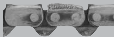
Worn PowerGRIT chain
