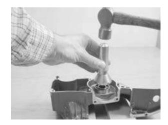
Install crankshaft into clutch side of case.
